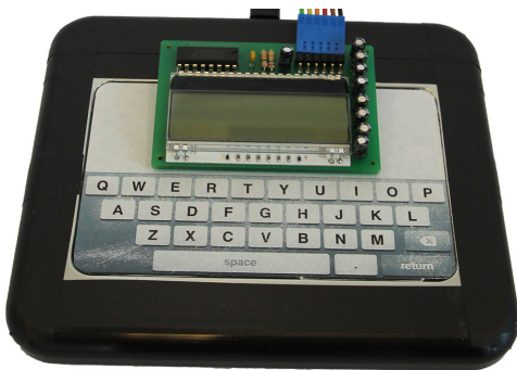
Figure 7. Modified Synaptics ForcePad used in the ForceType system.
